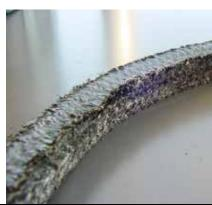
(left to right) Image 1. Extrusion of the seal material Image 2. Charred packing Image 3. Abraded packing (Images courtesy of the author)
