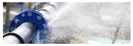
IMAGE 1: Improper gasket material selection and installation can lead to leaks (Image courtesy of Triangle Fluid Controls)
