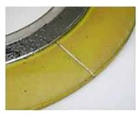
IMAGE 4: Grooves in four positions on outer ring of gasket prior to testing
