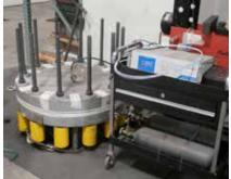
IMAGES 6 & 7: 75- and 360-ton test stands for ASME B16.20 test
