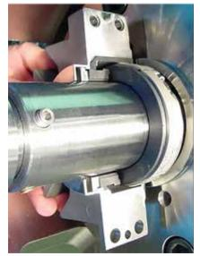
IMAGE 4: Split seal during installation (Image courtesy of Flowserve)
