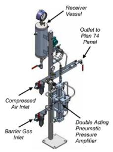
IMAGE 2: Typical pneumatic pressure amplifier with receiver vessel
