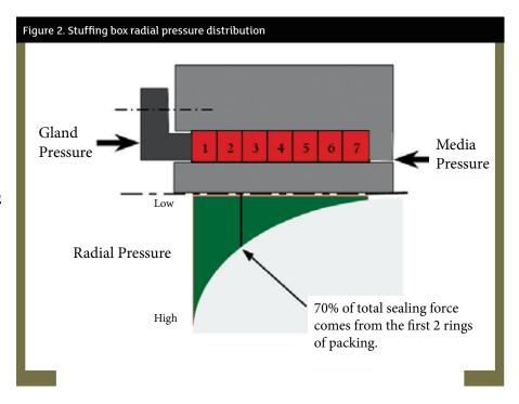
Keep checking the stuffing box temperature. A high temperature may indicate that the gland follower is overtightened. This can burn up the packing and damage the shaft or sleeve.
