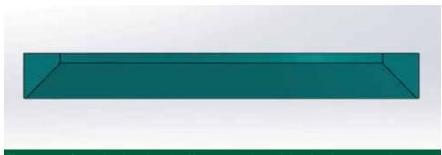
The structure of a metal seal consists of a wider top, an angle consisting of 45 degrees or 30 degrees and a wire-thin toe at the bottom.
