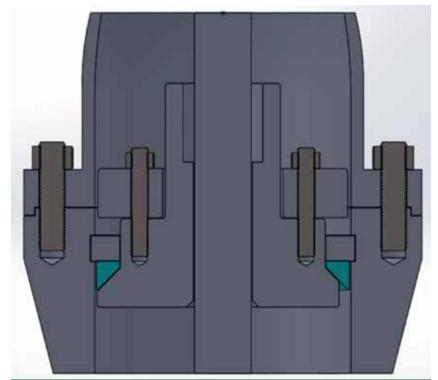
A pressure seal is a valve design that offers distinct advantages when compared to a conventional bolted body-to-bonnet sealing mechanism. It uses valve system pressure to keep thousands of pounds of pressure and system media contained within the valve.
