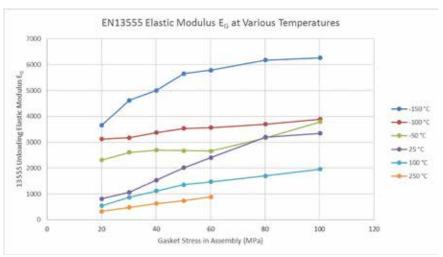
IMAGE 3: EN13555 elastic modulus at various temperatures
