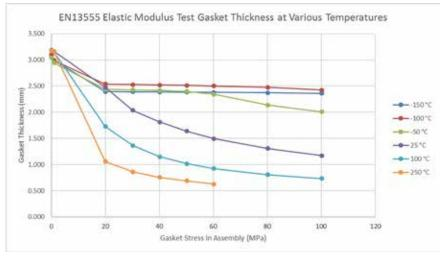
IMAGE 4: Elastic modulus test gasket thickness at various temperatures
