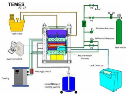
IMAGE 1: Testing device for cooling system (Images courtesy of FSA)
