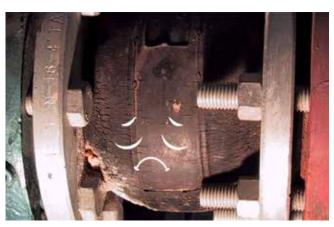
IMAGE 5: Hard-boiled expansion joint
