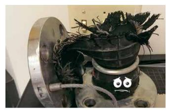
IMAGE 4: Failed expansion joint
