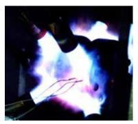
IMAGE 4: Exxon-modified API 607 gasket fire test
