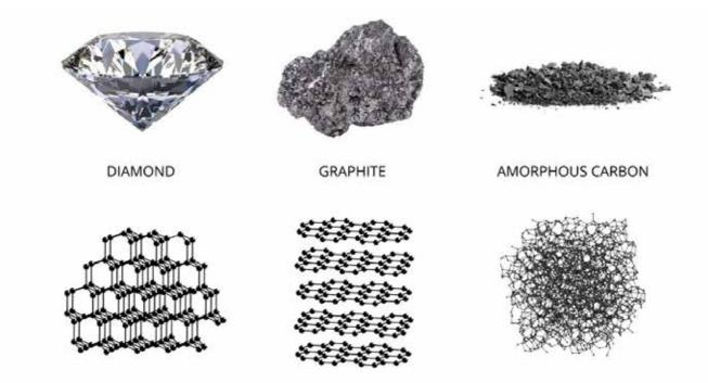
IMAGE 2: Carbon exists in three forms in nature—diamond, graphite and amorphous carbon. Diamond: Four bonded valence electrons. Highly ordered lattice structure. Graphite: Three bonded valence electrons. Strong graphene layers bound together by weak van der Waals forces. Amorphous Carbon: Two bonded valence electrons. Strong "entanglement" of carbons.
